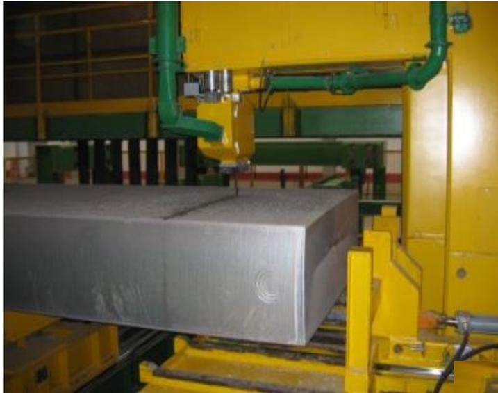
*Slab sawing (head + foot cut)*
