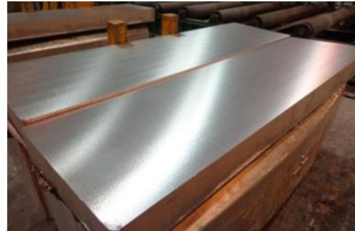
*Slab sawing (head + foot cut)*
