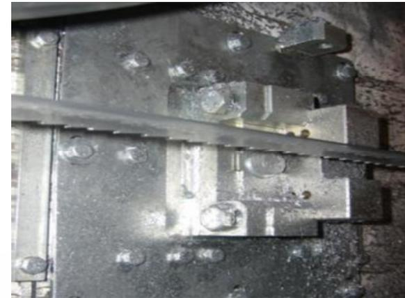
b) Long bracket and support for slicing saws
