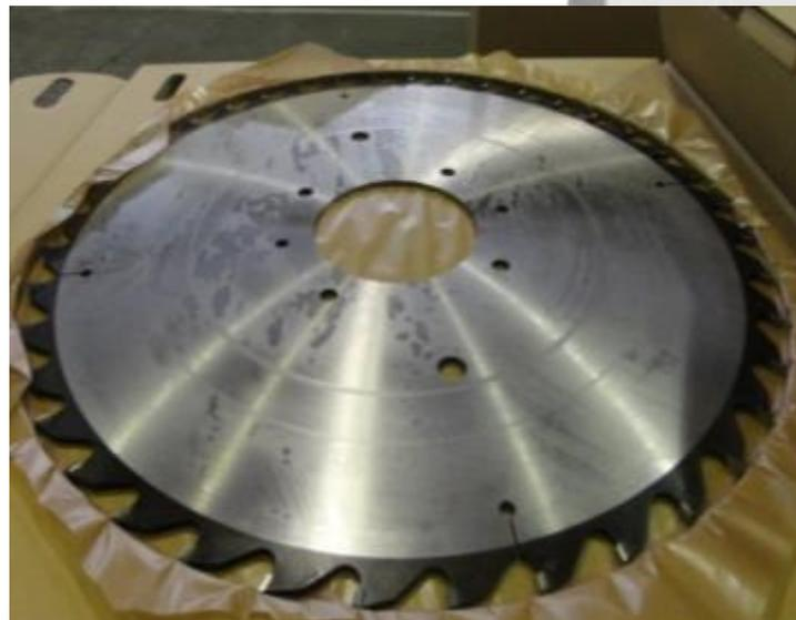
*TCT saw-blades of diameters 950mm and 860mm
